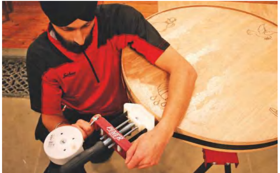
▲ Pic.16 Securing the lath in place using a band clamp
